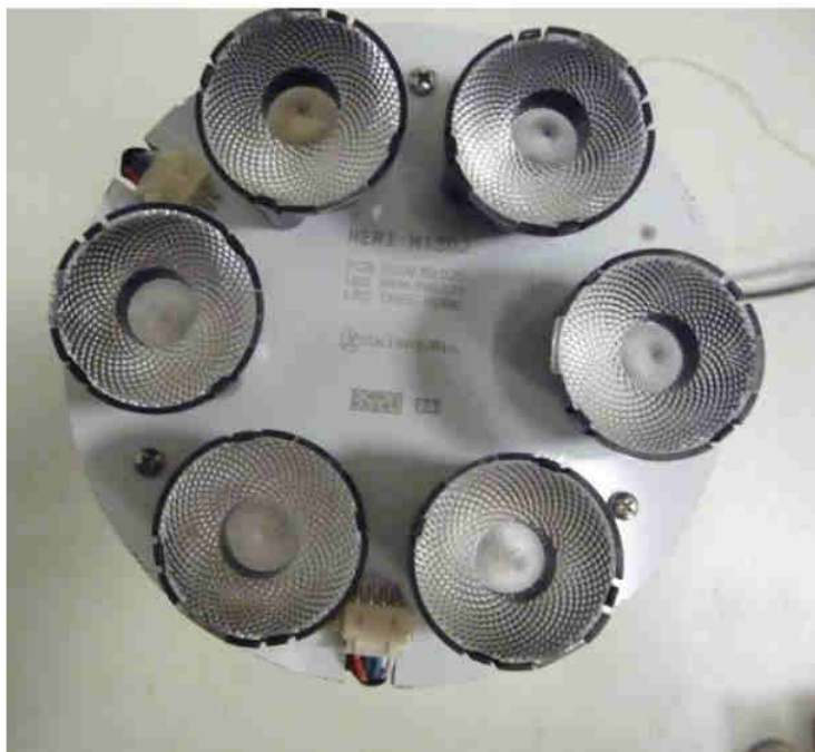
Photograph No. 12 Plastic lenses over LED modules NEBULA RGBW
