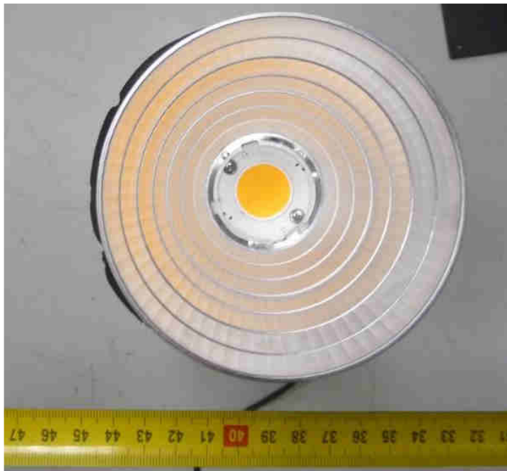
Photograph No. 11 Reflector over COB LED in NEBULA PR
