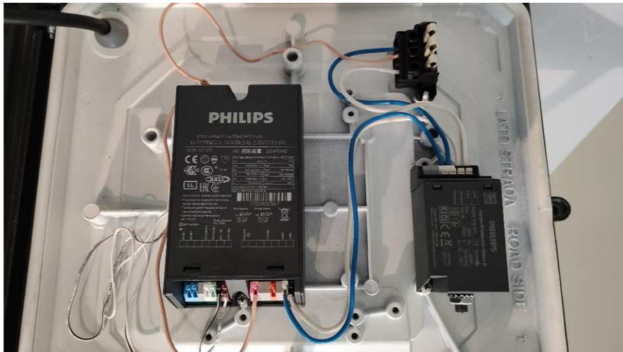
Photograph No. 4. LED controlgear
