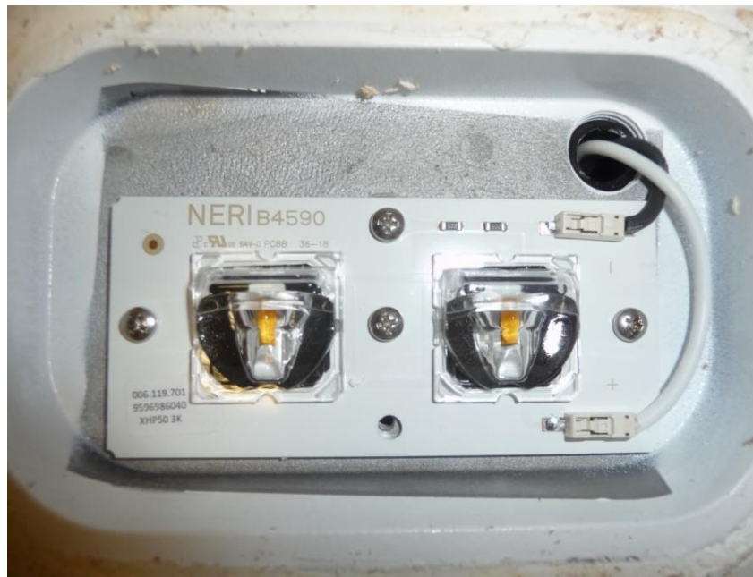
Photograph No. 6 View of the LED module (2 LEDs)
