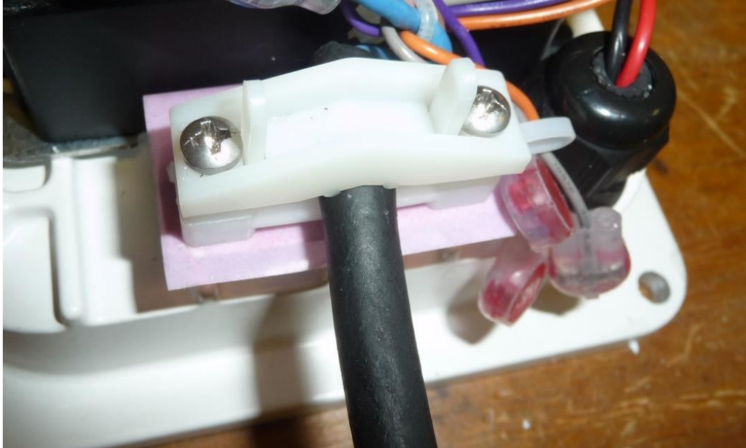
Photograph No. 7 Connections and cord anchorage
