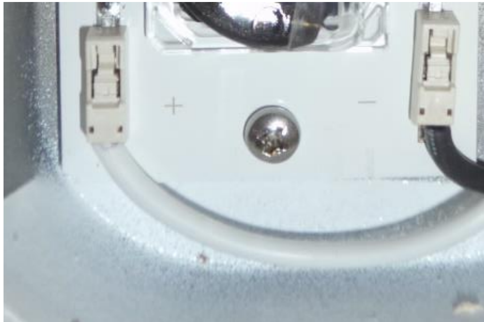
Photograph No. 8 LED module supply terminals
