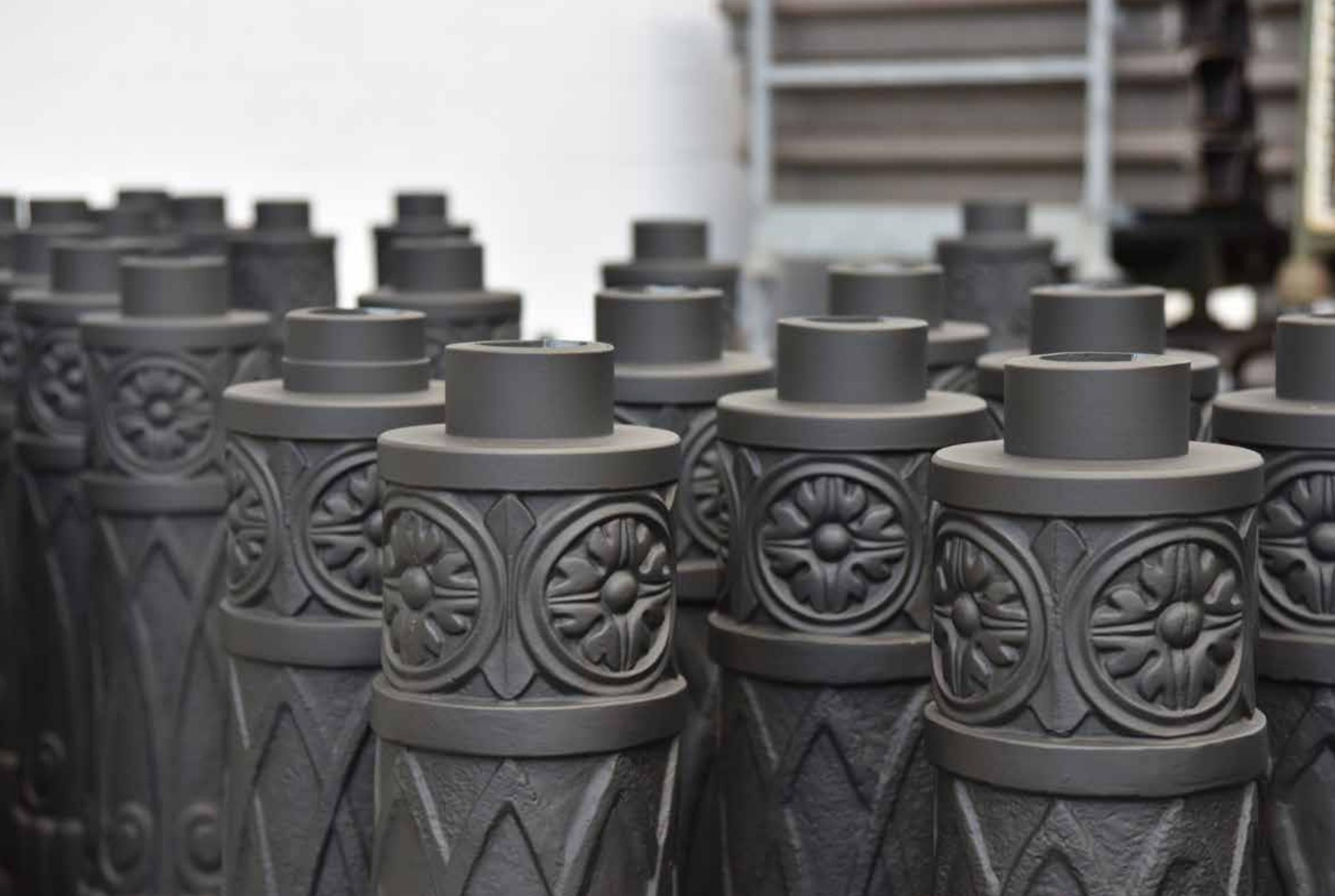
The furnishing of the Royal Gardens also included a number of slender, elegant lamp posts. It was necessary to cast 9 new ones, for which the foundry set up a model derived from the best conserved exemplar. Here, too, a core had to be designed and formed to create the hollow interior. This was a highly complex operation on account of the notable length of the model.
