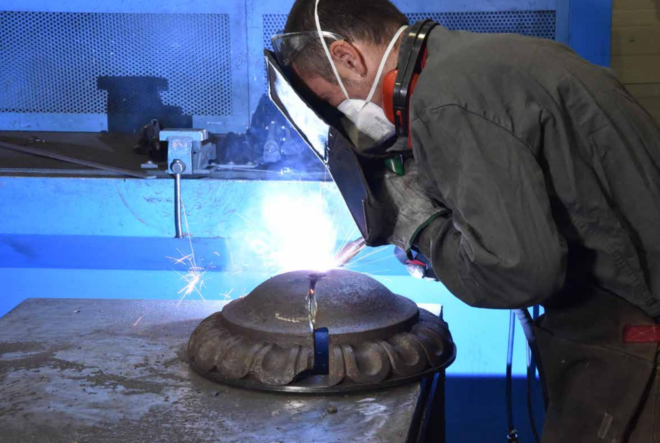
Not all the parts had been saved, however. Four were missing or were irretrievably broken. As with the other parts, the best conserved items were chosen and used as a model for new castings.
