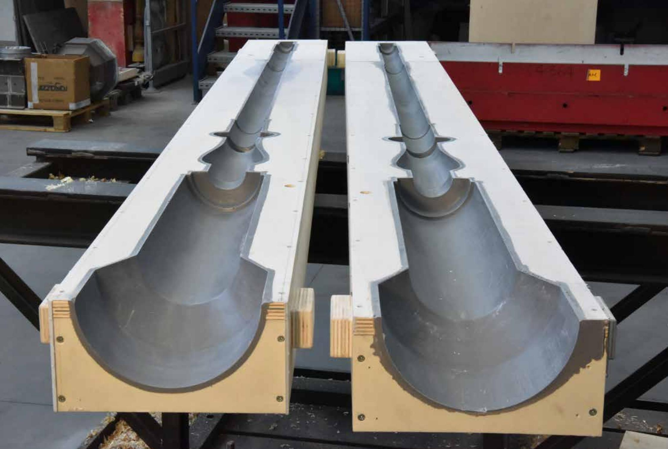
The casting pattern for the lamp posts, including the lateral decorations and the hollow interior, was obtained in the foundry with great mastery and much patient manual work. Finally, the cast iron was poured into the shaft containing the mold for the lamp post. A long process that had to be performed 9 times over.
