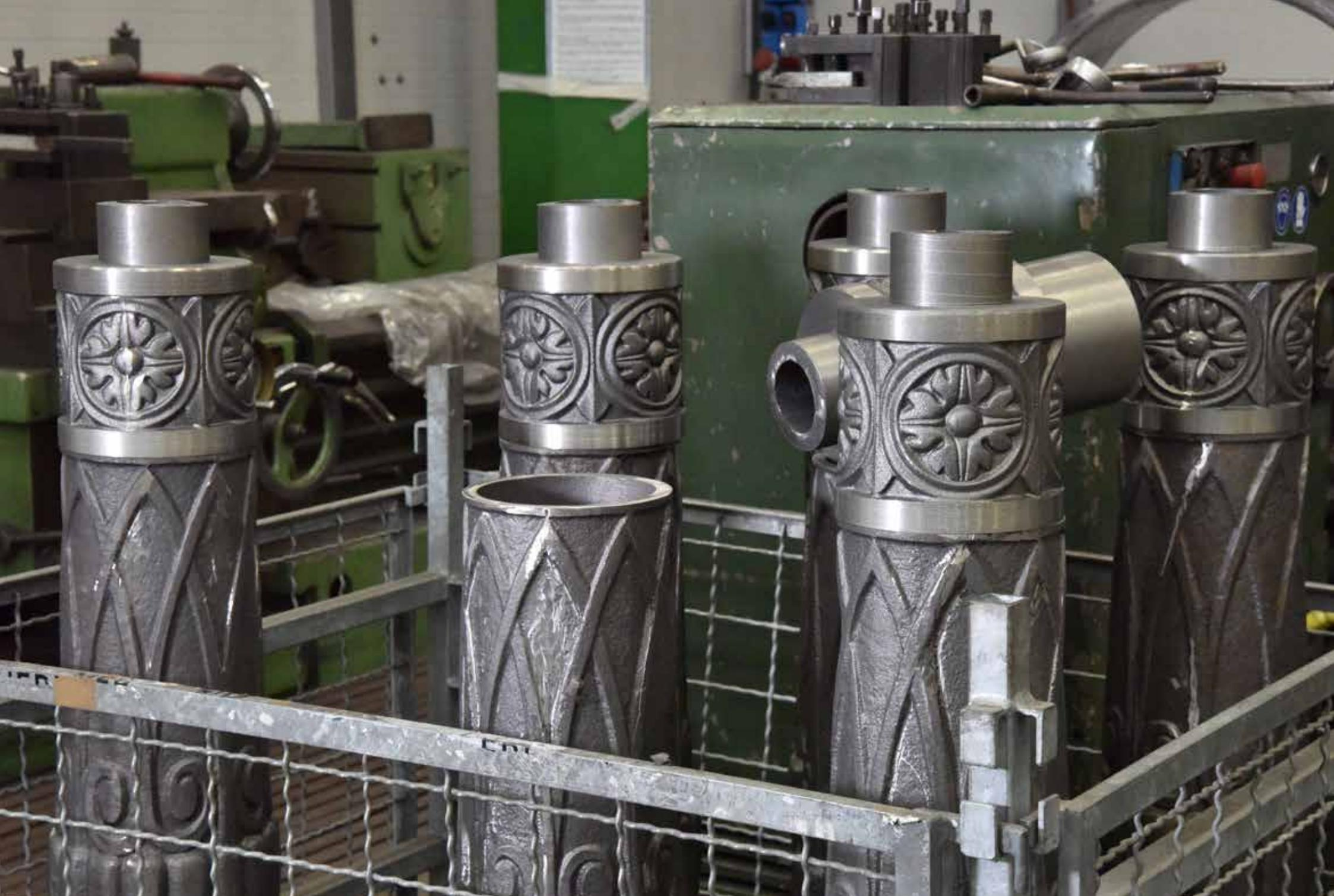
Some of the columns were irredeemably compromised and a new model had to be created to reproduce them. The best conserved column was chosen and equipped with lateral “gates” in wood to allow the casting. Lastly, the “core box”, which reproduces perfectly the inner form of the column, was created. Using the external model and the core box, the parts needed to complete the pergola could be cast.
