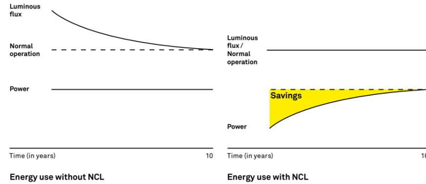
The light output of the system is kept consistent throughout the life of the product by acting on the current supplied and compensating for the decay of the source.
