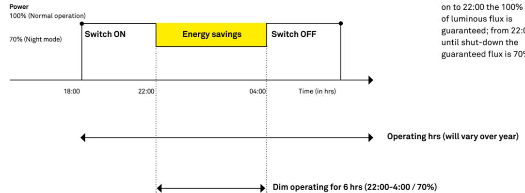
Dimming preset cycle: from the switching on to 22:00 the 100% of luminous flux is guaranteed; from 22:00 until shut-down the guaranteed flux is 70%.
