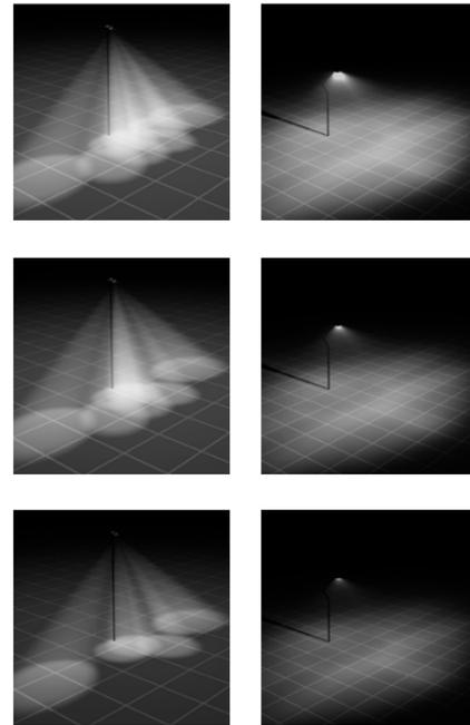
On the left, from top to bottom, diagrammatic views of LEDs without multilayer lenses.
