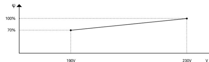
Example of AmpDim setting: with a feed voltage of 230V, the product is at 100% of its flux; the flux regulator reduces the feed voltage to 190V, thus reaching 70% of its flux.
