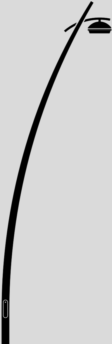
Alkes post top luminaire with arm curved conical post with arm h 7 and 8 m, lighting product Light 34
