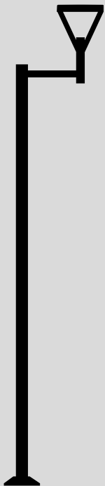
Post top luminaires with arm Lyra h 12'
